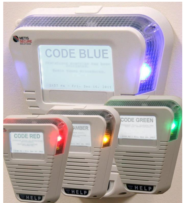
MS-5100 Emergency Help Stations display color-coded messages and lights to maximize response at VeriSign.
